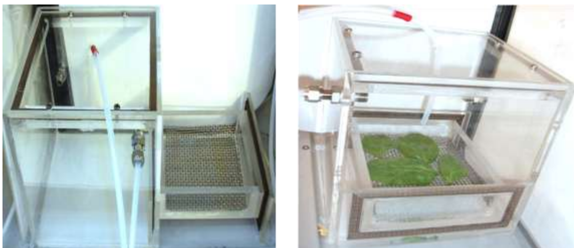
Figure 12: Modified ozone fumigation system
